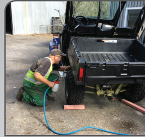
Chassis coated with Prolan – No corrosion
